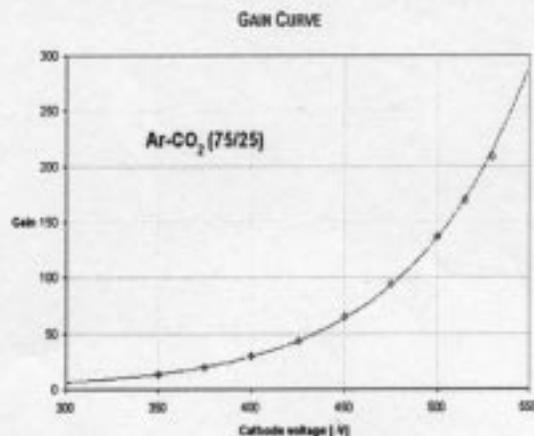
**Figure 7** Apparent gas gain as a function of cathode voltage.
