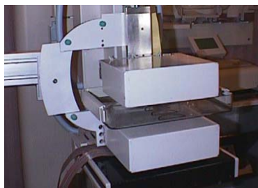
Figure VI-9: Jefferson Lab positron emission mammography (PEM) system used to image metabolically active breast tumors at Duke University Medical Center, shown integrated with an X-ray mammography system.
